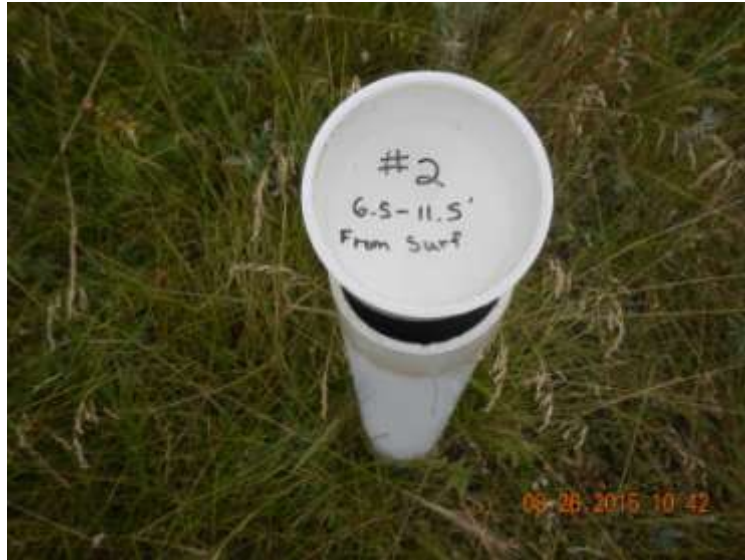
Monitoring Well (MW) #2 – 4” PVC pipe approximately 2.5’ above ground surface. No hydrocarbon odor.
