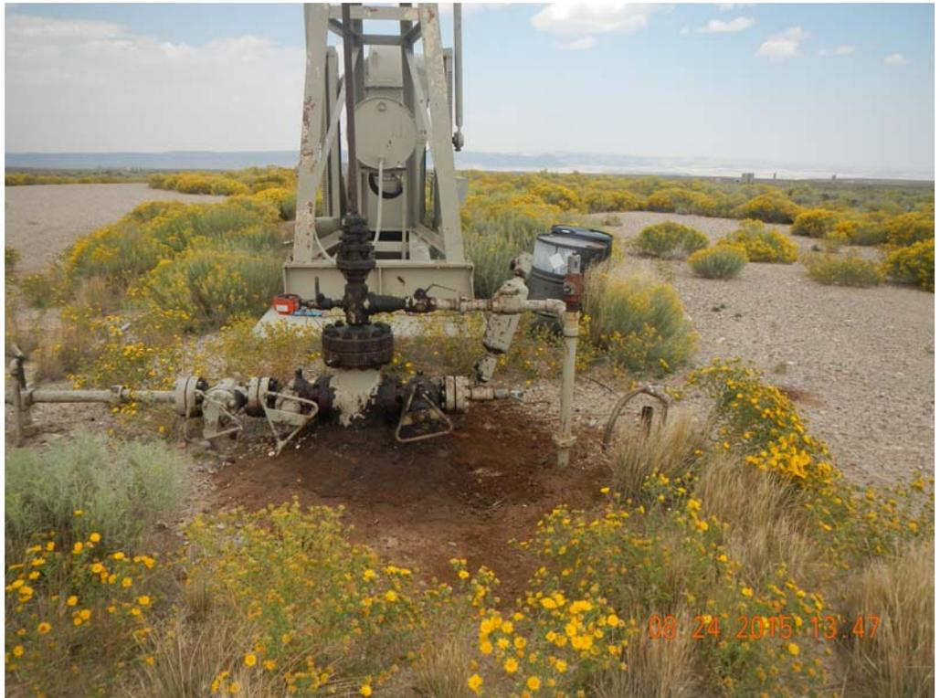
No wellhead sign. Lube oil stored at wellhead with no secondary containment.
