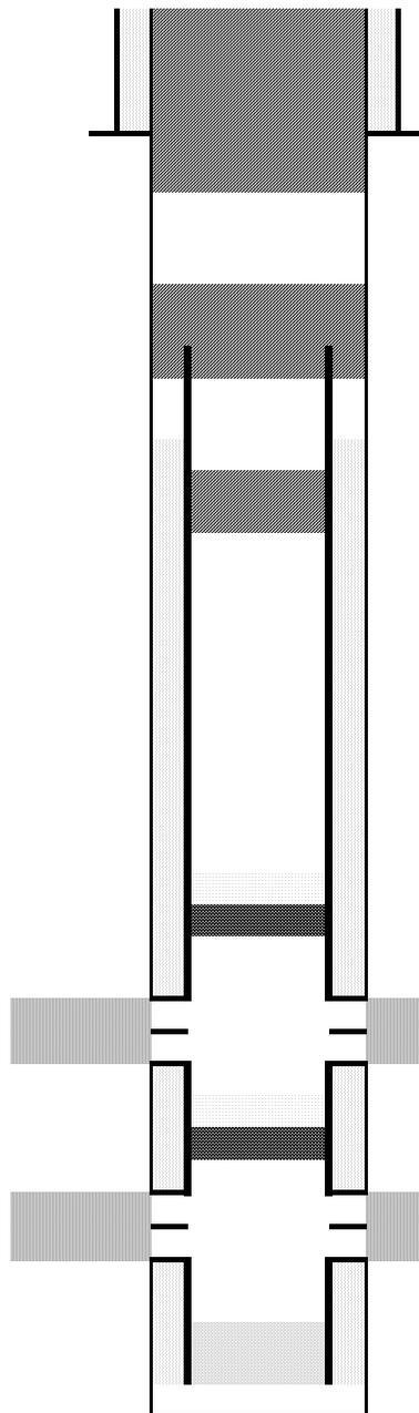
Cut surface casing off 6'-8' below surface.
