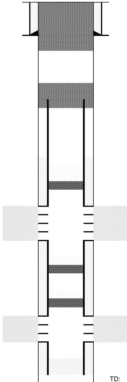
Cut surface casing off 6'-8' below surface.
