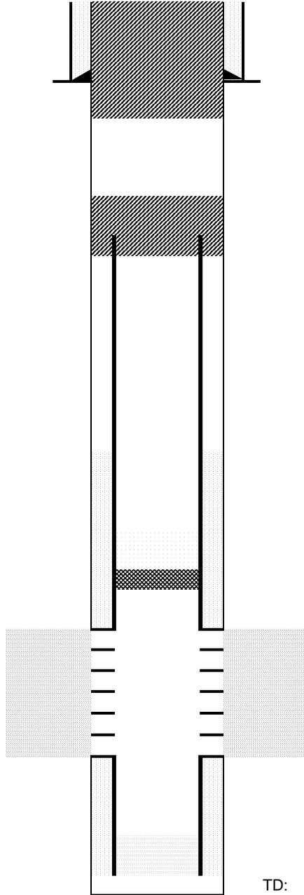
Cut surface casing off 6'-8' below surface.
