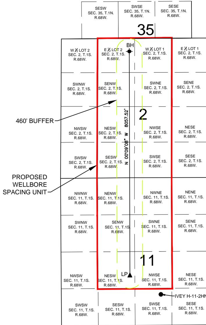
**WELL IVEY H-11-2HN TO BE LOCATED 1105' FSL AND 1720' FEL, SEC. 11, T1S, R68W**
