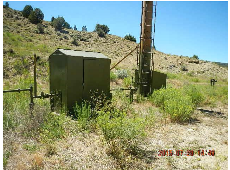
Tank battery sign – incomplete. Weeds/brush within 25' of production equipment.
