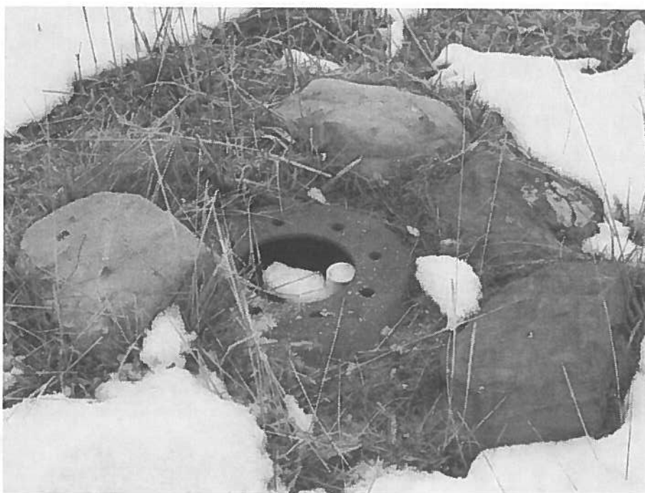
Photo 7: Permanent soil vapor monitoring probe next to Phillip J. Schalles #1 abandoned well marker.
