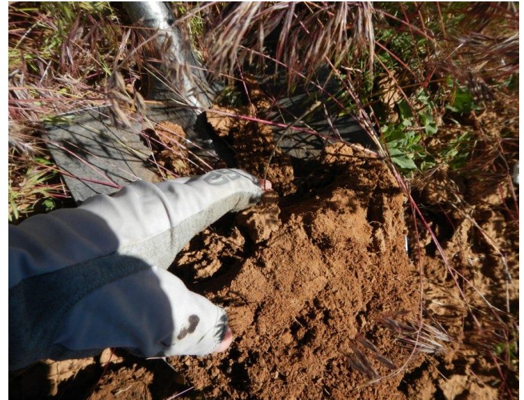
Photos 3 and 4. Close-up view of soil from well pad that is compacted (on left) and close-up of soil outside of the project area that is loose and not compacted ( on right).
