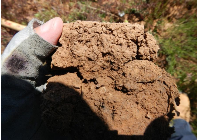
Photos 3 and 4. Close-up view of soil from well pad that is compacted (on left) and close-up of soil outside of the project area that is loose and not compacted ( on right).
