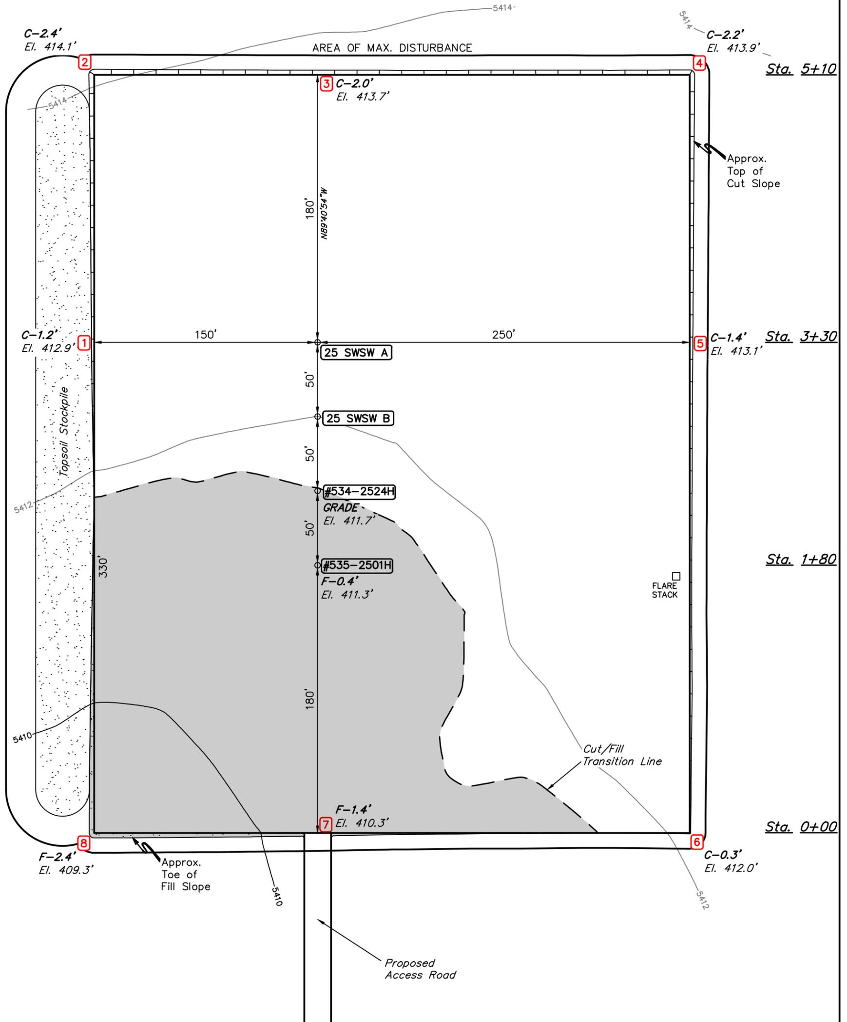
NOTE: Earthwork Calculations Require a Fill @ Some of the Location Stakes For Balance. All Fill is to be Compacted to a Minimum of 95% of the Maximum Dry Density Obtained by AASHTO Method t-99.
