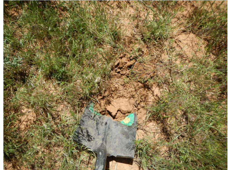
Photo 5. View of non-compacted soils outside of project area (photo on right). Soil is soft and easy to dig in. Photo is taken approximately 50 feet south of location in adjacent pasture.
