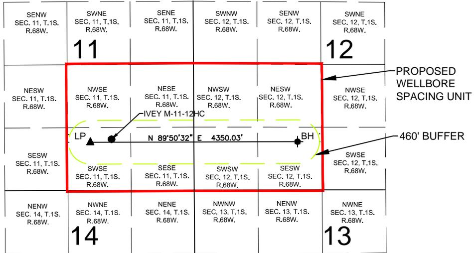
WELL **IVEY M-11-12HC** TO BE LOCATED 1077' FSL AND 1730' FEL, SEC. 11, T1S, R68W
