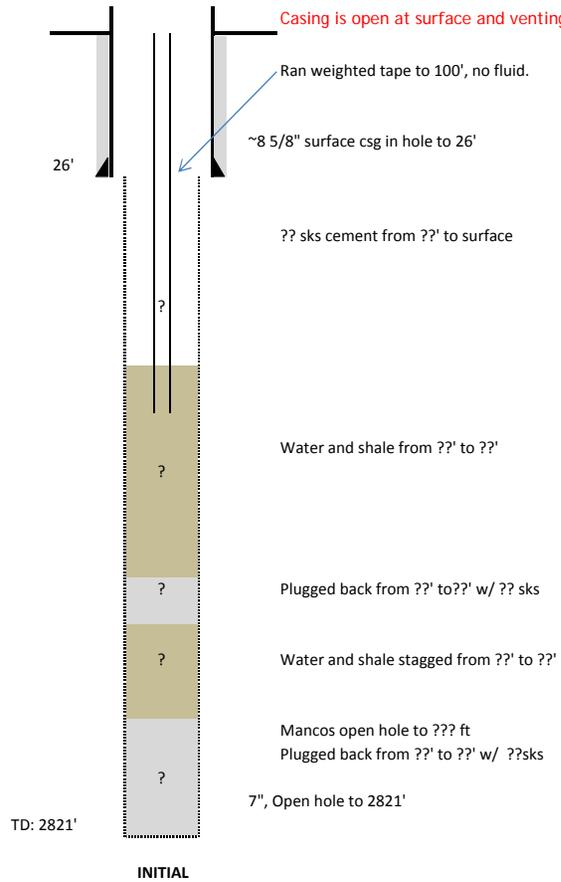
Casing is open at surface and venting methane. Tubing in casing.
