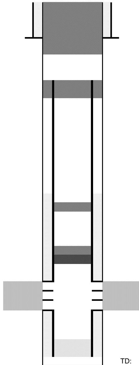
Cut surface casing off 6'-8' below surface.
