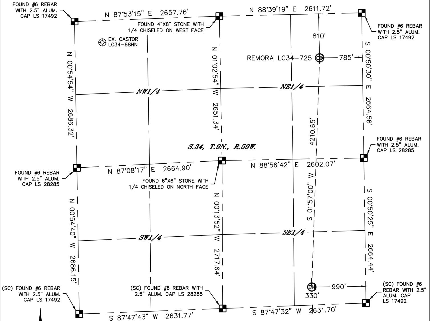
In accordance with a request from Brian James with Noble Energy Inc. Lat40°, Inc. has determined the surface location of the REMORA LC34-725 to be 810' from the NORTH line and 785' from the EAST line and the bottom hole to be 330' from the SOUTH line and 990' from the EAST line as measured at right angles from the section lines of Section 34, Township 9 North, Range 59 West of the Sixth Principal Meridian, County of Weld, State of Colorado.
