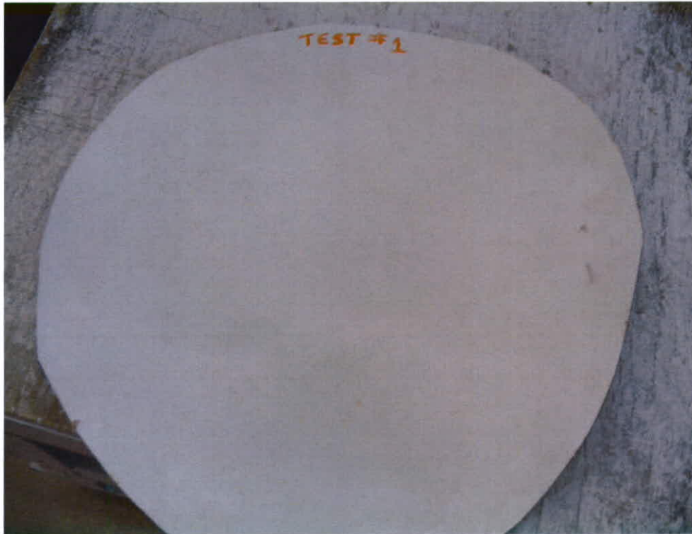
Test No. 1 geomembrane post exposure
