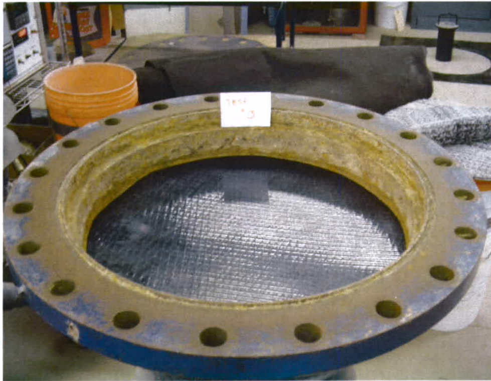
Test No. 3 geomembrane post exposure
