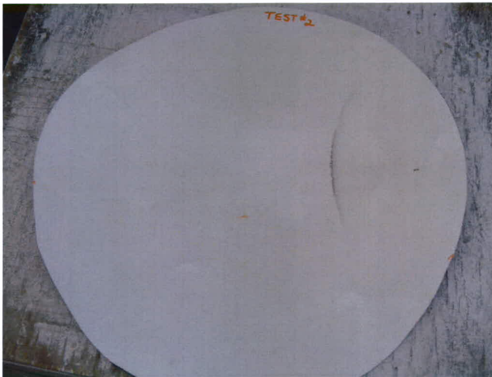
Test No. 2 geomembrane post exposure
