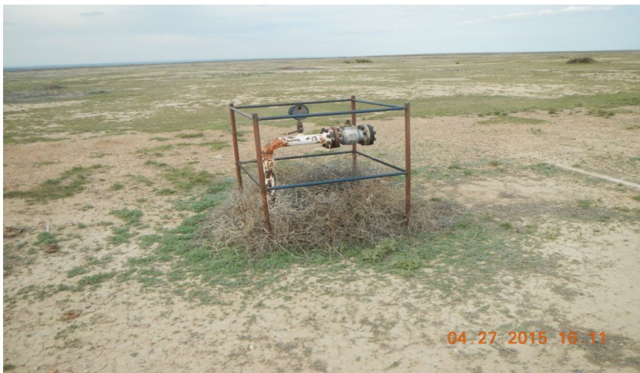
photo 10: Pipe riser at center of location. Lat/Long:37.95993,-102.50062.
