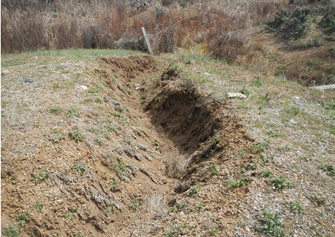
Photo 6. View of an erosional channel in the southeastern corner of the project area flowing toward the eastern wetland complex. This channel is approximately 2 to 3 feet wide and 4 feet deep.
