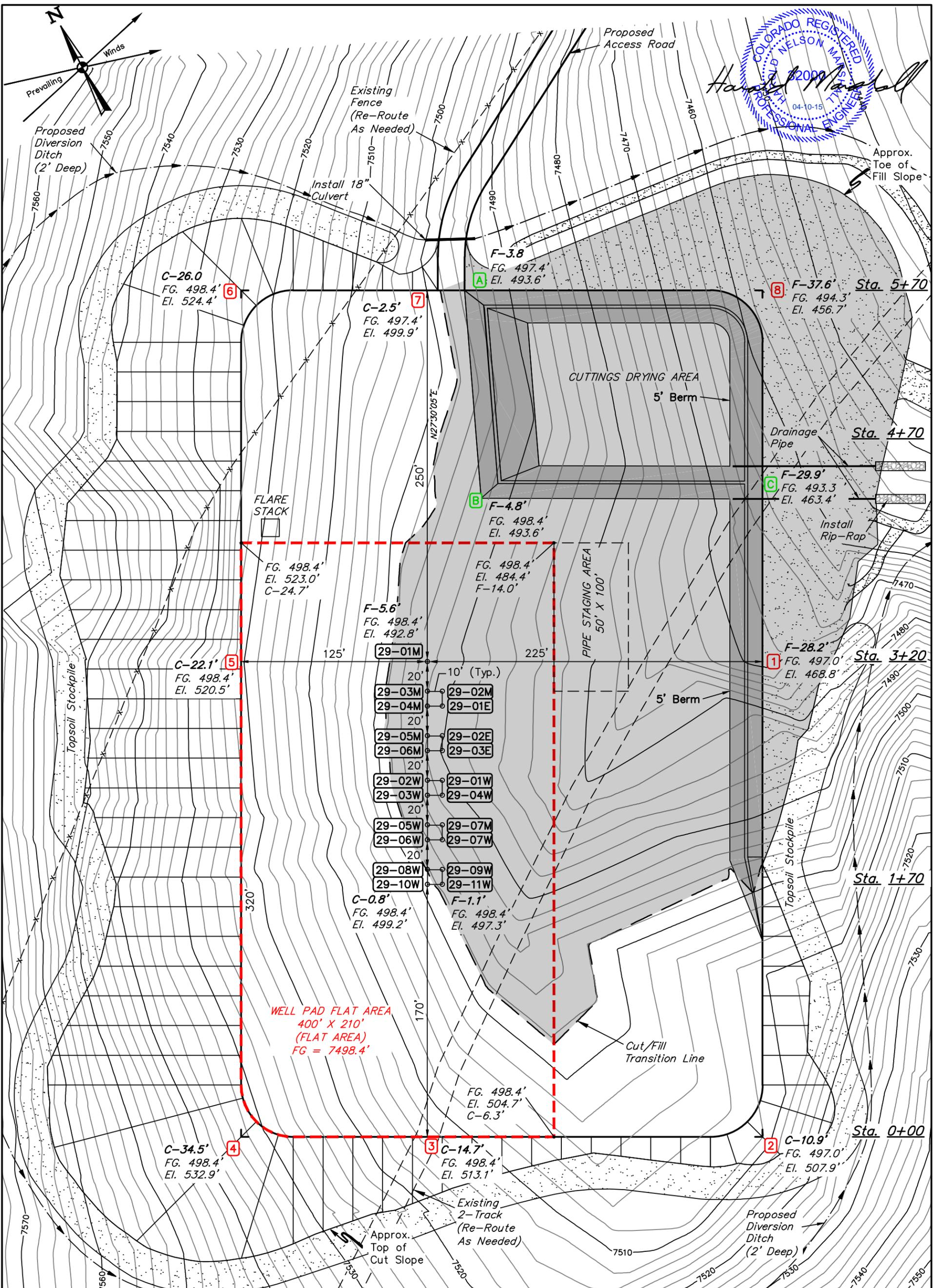
**FINISHED GRADE ELEVATION OF WELL PAD FLAT AREA = 7498.4'**
