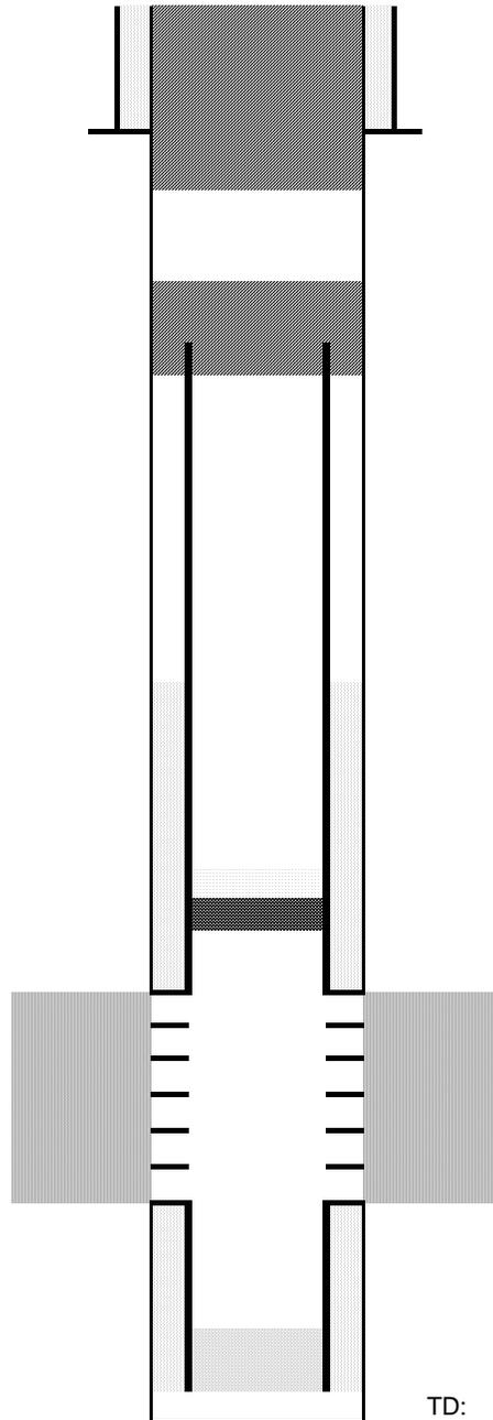
Cut surface casing off 6'-8' below surface.
