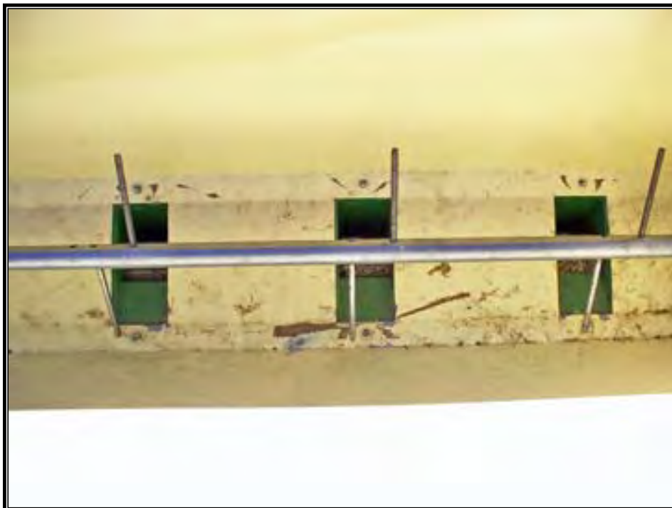
Photo 18: Small Grain Standard Seed Box/Seed Cups
