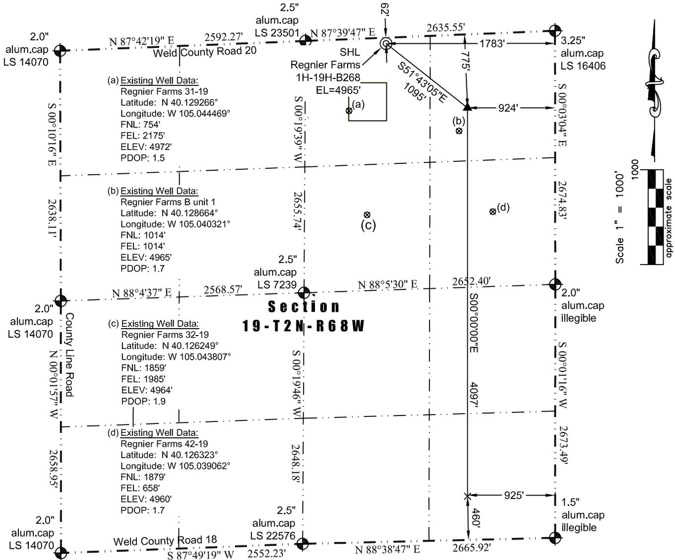
In accordance with a request from Jay Knutson of EnCana Oil & Gas (USA) Inc., Washburn Land Surveying, LLC has determined the location of the **Regnier Farms 1H-19H-B268** well site to be SHL: 62' FNL and 1783' FEL, (TPZ: 775' FNL and 924' FEL), (BHL: 460' FSL and 925' FEL), as measured at ninety (90) degrees from the section lines of Section 19 Township 2 North, Range 68 West of the 6th Principal Meridian, Weld County Colorado.
