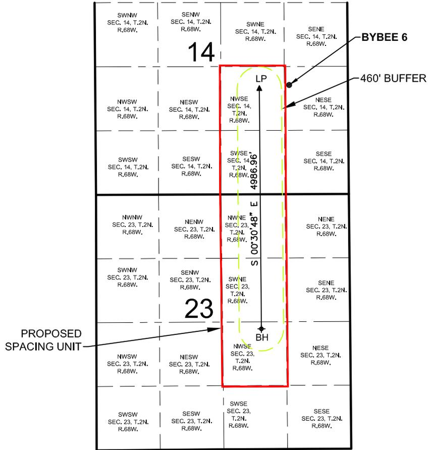
**WELL BYBEE 6 TO BE LOCATED 2268' FSL AND 1220' FEL, SEC. 14, T2N, R68W**
