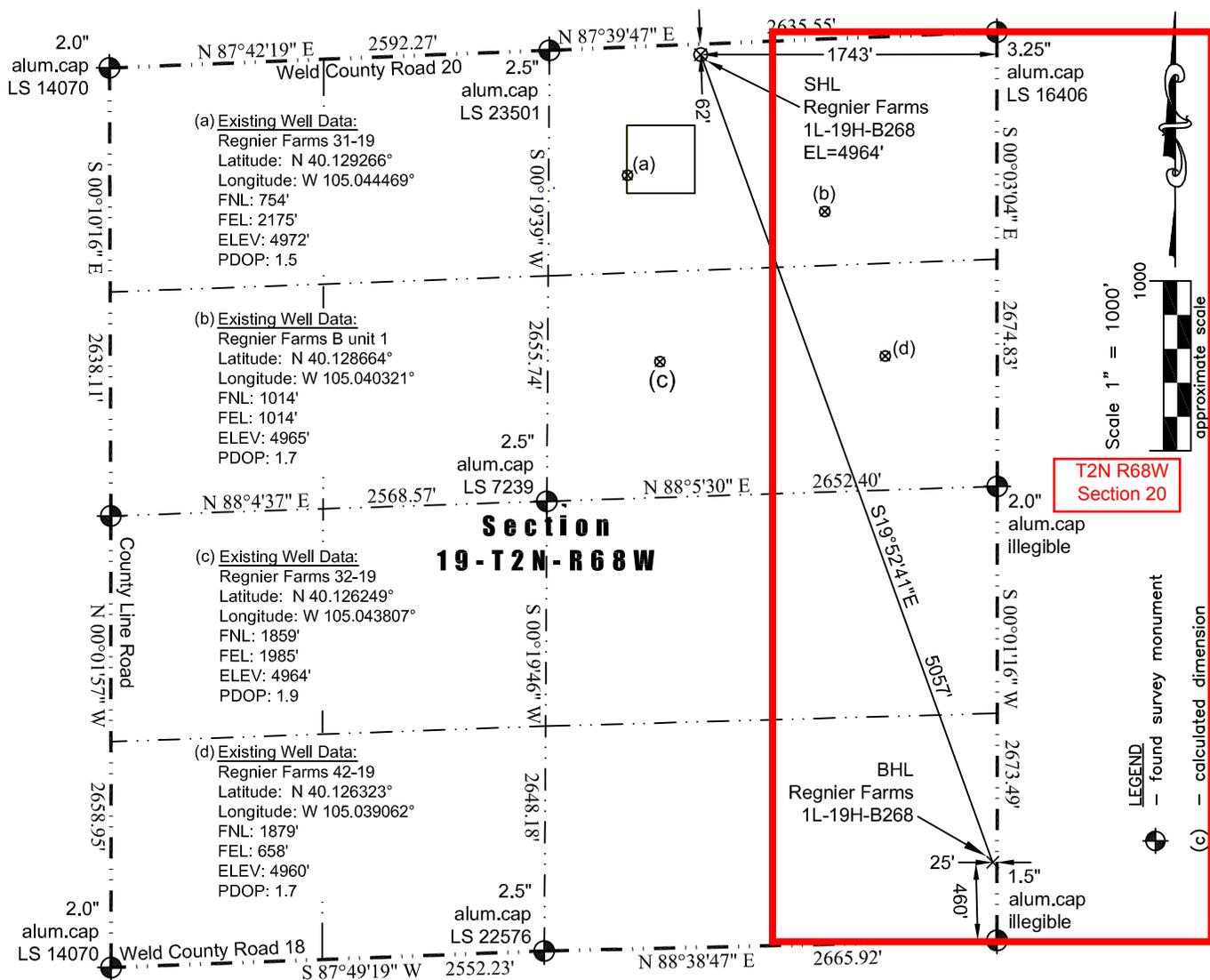
In accordance with a request from Jay Knutson of EnCana Oil & Gas (USA) Inc., Washburn Land Surveying, LLC has determined the location of the **Regnier Farms 1L-19H-B268** well site to be SHL: 62' FNL and 1743' FEL, (BHL: 460' FSL and 25' FEL), as measured at ninety (90) degrees from the section lines of Section 19 Township 2 North, Range 68 West of the 6th Principal Meridian, Weld County Colorado.
