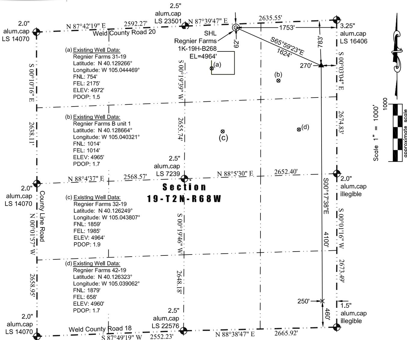
In accordance with a request from Jay Knutson of EnCana Oil & Gas (USA) Inc., Washburn Land Surveying, LLC has determined the location of the **Regnier Farms 1K-19H-B268** well site to be SHL: 62' FNL and 1753' FEL, (TPZ: 783' FNL and 270' FEL), (BHL: 460' FSL and 250' FEL), as measured at ninety (90) degrees from the section lines of Section 19 Township 2 North, Range 68 West of the 6th Principal Meridian, Weld County Colorado.
