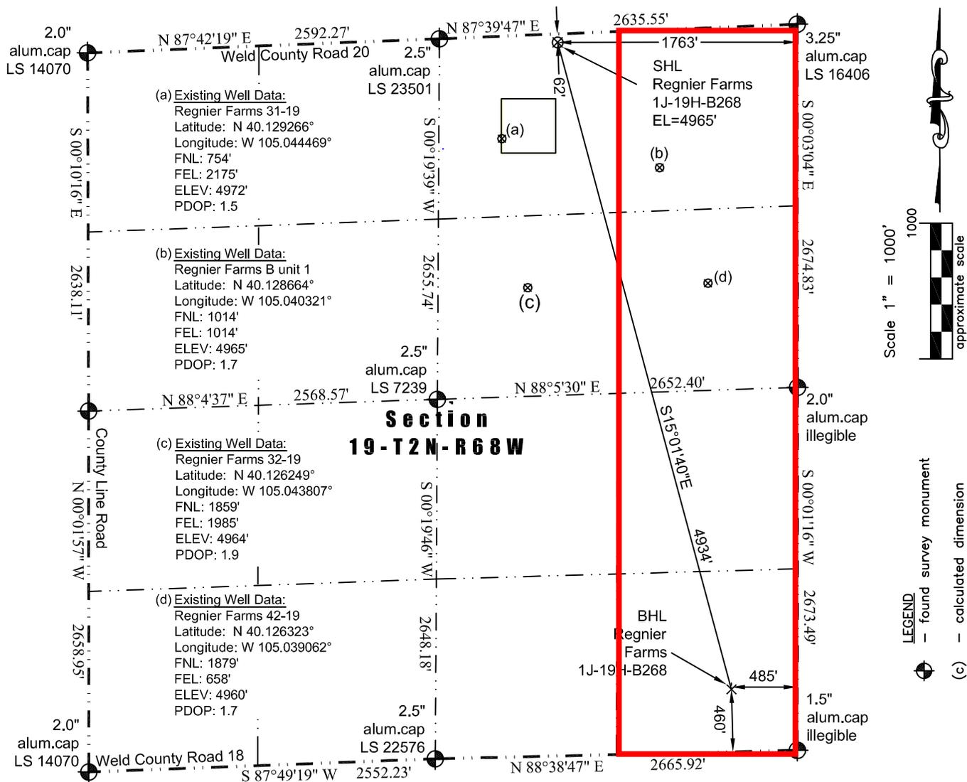
In accordance with a request from Jay Knutson of EnCana Oil & Gas (USA) Inc., Washburn Land Surveying, LLC has determined the location of the **Regnier Farms 1J-19H-B268** well site to be SHL: 62' FNL and 1763' FEL, (BHL: 460' FSL and 485' FEL), as measured at ninety (90) degrees from the section lines of Section 19 Township 2 North, Range 68 West of the 6th Principal Meridian, Weld County Colorado.
