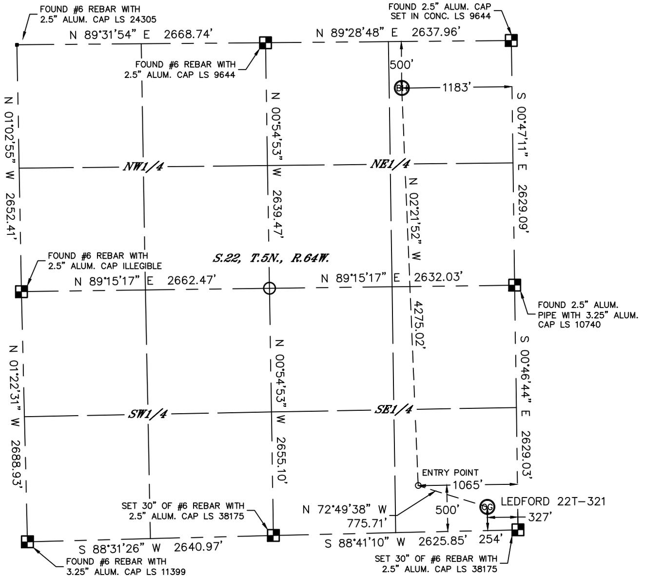
In accordance with a request from Jake Bragg with PDC ENERGY Lat40°, Inc. has determined the surface location of the LED FORD 22T-321 to be 254' from the SOUTH line and 327' from the EAST line and the bottom hole to be 500' from the NORTH line and 1183' from the EAST line as measured at right angles from the section lines of Section 22, Township 5 North, Range 64 West of the Sixth Principal Meridian, County of Weld, State of Colorado.
