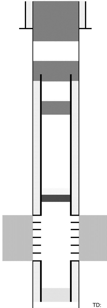
Cut surface casing off 6'-8' below surface.
