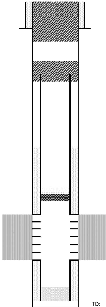
Cut surface casing off 6'-8' below surface.
