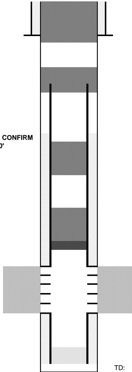
Cut surface casing off 6'-8' below surface.
