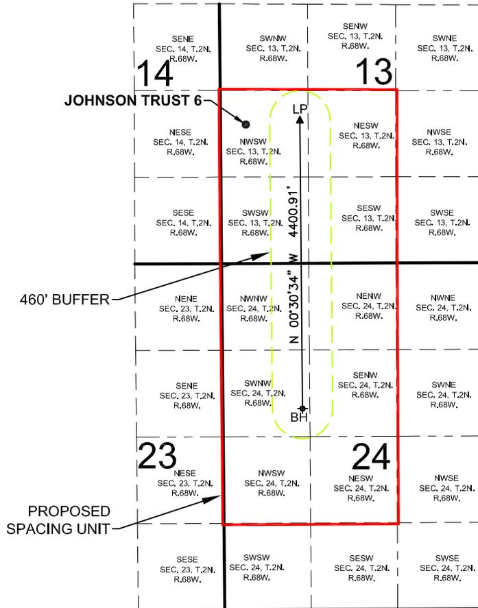
**WELL JOHNSON TRUST 6 TO BE LOCATED 2125' FSL AND 388' FWL, SEC. 13, T2N, R68W**
