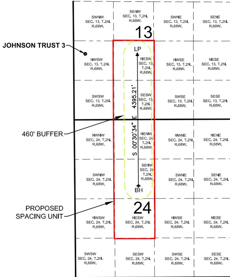
WELL **JOHNSON TRUST 3** TO BE LOCATED 2209' FSL AND 389' FWL, SEC. 13, T2N, R68W
