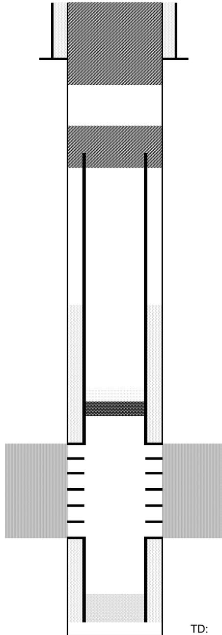
Cut surface casing off 6'-8' below surface.
