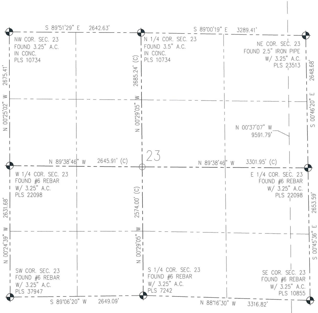
**N** IN ACCORDANCE WITH A REQUEST FROM CRAIG RASMUSON - SYNERGY RESOURCES, BASELINE ENGINEERING CORP. HAS DETERMINED THE LOCATION OF THE SRC EVANS 43-26-23-14NHZ TO BE 1890' FNL AND 2130' FEL, AS MEASURED AT NINETY (90) DEGREES FROM THE SECTION LINE OF SECTION 26, TOWNSHIP 5 NORTH, RANGE 66 WEST AND THE BOTTOM HOLE LOCATION TO BE 2162' FSL AND 350' FEL OF SECTION 14, TOWNSHIP 5 NORTH, RANGE 66 WEST, 6TH PRINCIPAL MERIDIAN, WELD COUNTY, COLORADO.
