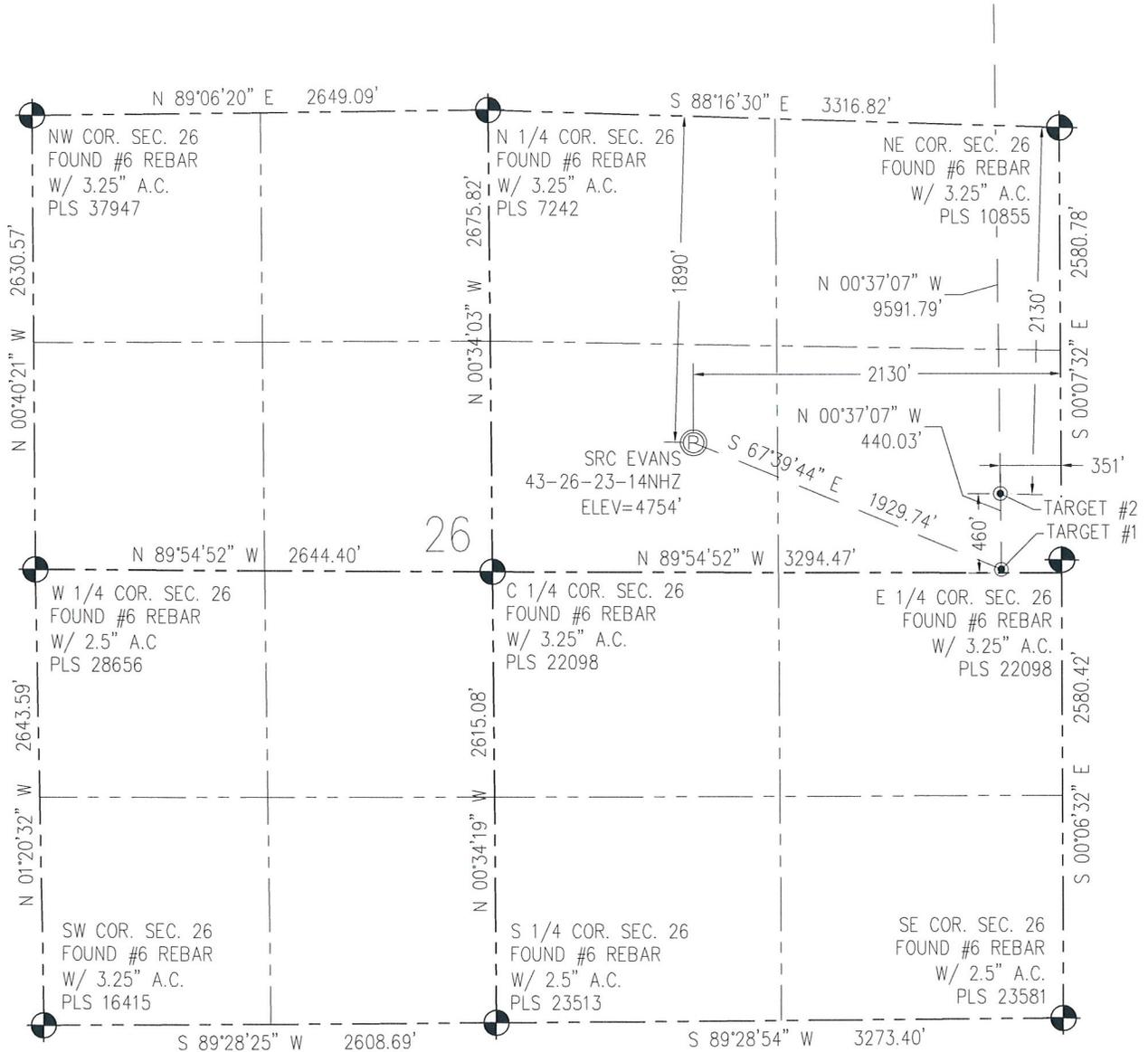
IN ACCORDANCE WITH A REQUEST FROM CRAIG RASMUSON - SYNERGY RESOURCES, BASELINE ENGINEERING CORP. HAS DETERMINED THE LOCATION OF THE SRC EVANS 43-26-23-14NHZ TO BE 1890' FNL AND 2130' FEL, AS MEASURED AT NINETY (90) DEGREES FROM THE SECTION LINE OF SECTION 26, TOWNSHIP 5 NORTH, RANGE 66 WEST AND THE BOTTOM HOLE LOCATION TO BE 2162' FSL AND 350' FEL OF SECTION 14, TOWNSHIP 5 NORTH, RANGE 66 WEST, 6TH PRINCIPAL MERIDIAN, WELD COUNTY, COLORADO.
