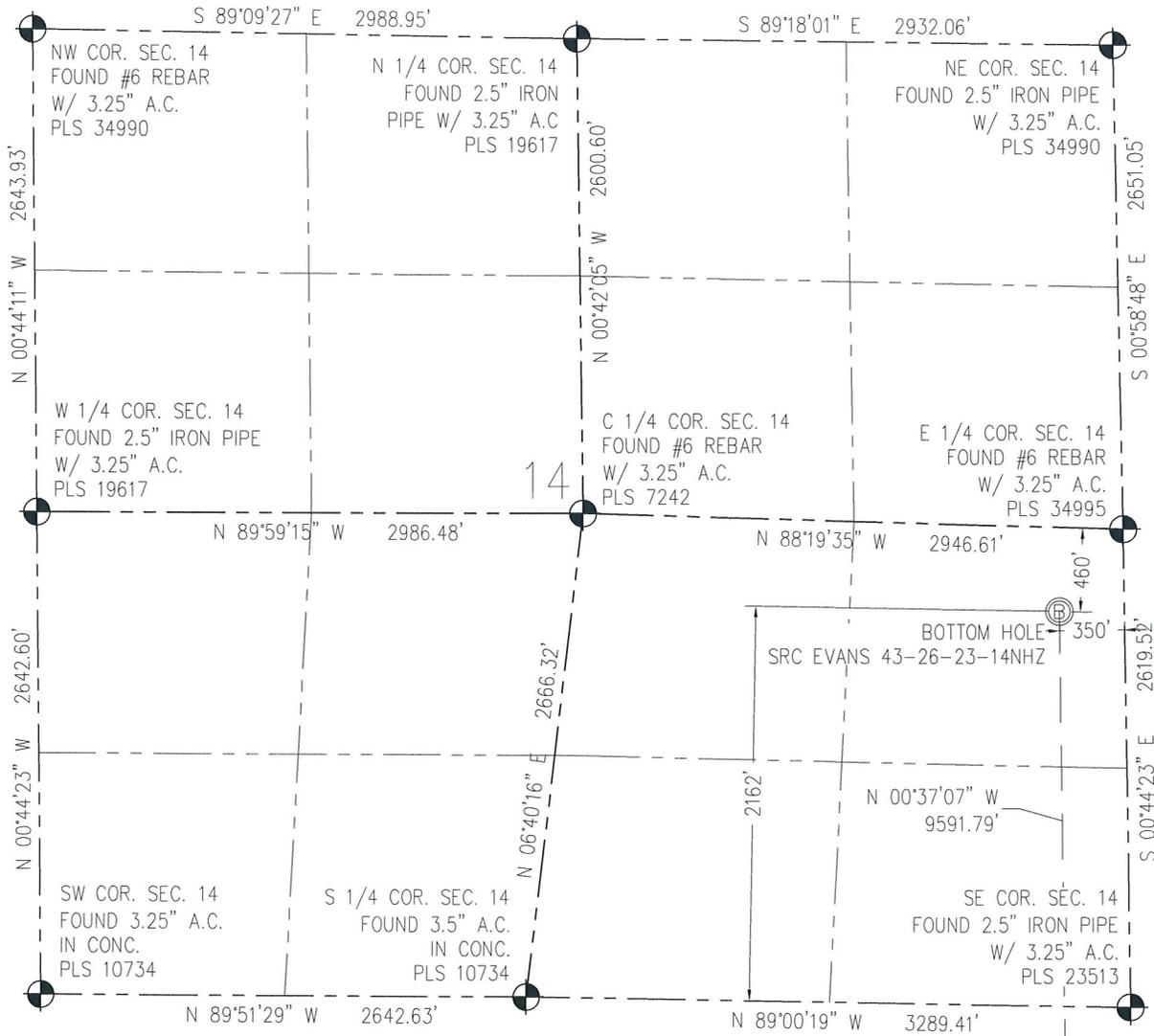
**N** IN ACCORDANCE WITH A REQUEST FROM CRAIG RASMUSON - SYNERGY RESOURCES, BASELINE ENGINEERING CORP. HAS DETERMINED THE LOCATION OF THE SRC EVANS 43-26-23-14NHZ TO BE 1890' FNL AND 2130' FEL, AS MEASURED AT NINETY (90) DEGREES FROM THE SECTION LINE OF SECTION 26, TOWNSHIP 5 NORTH, RANGE 66 WEST AND THE BOTTOM HOLE LOCATION TO BE 2162' FSL AND 350' FEL OF SECTION 14, TOWNSHIP 5 NORTH, RANGE 66 WEST, 6TH PRINCIPAL MERIDIAN, WELD COUNTY, COLORADO.
