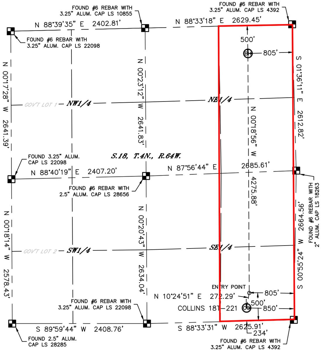
In accordance with a request from Steve Tracy with PDC ENERGY Lat40°, Inc. has determined the surface location of the COLLINS 18T-221 to be 234' from the SOUTH line and 850' from the EAST line and the bottom hole to be 500' from the NORTH line and 805' from the EAST line as measured at right angles from the section lines of Section 18, Township 4 North, Range 64 West of the Sixth Principal Meridian, County of Weld, State of Colorado.
