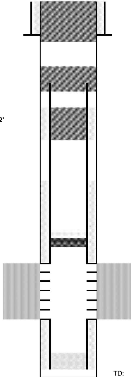
Cut surface casing off 6'-8' below surface.
