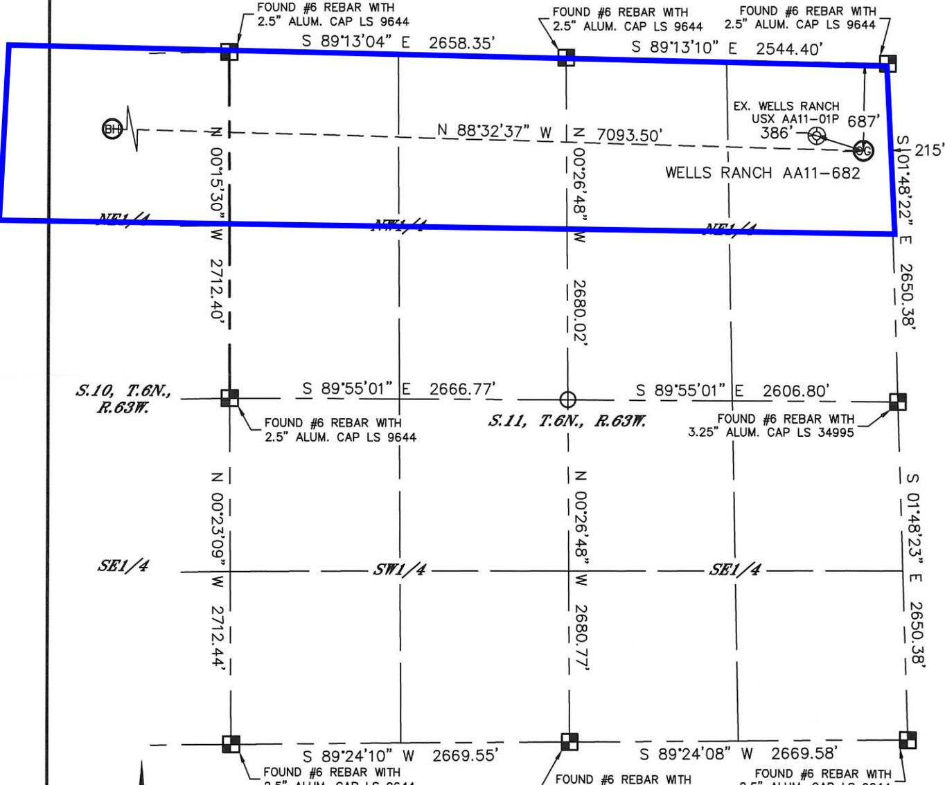
In accordance with a request from Greg Wilson with Noble Energy Inc. Lat40, Inc. has determined the surface location of the WELLS RANCH AA11-682 to be 687' from the NORTH line and 215' from the EAST line of Section 11, Township 6 North, Range 63 West and the bottom hole to be 535' from the NORTH line and 2085' from the EAST line as measured at right angles from the section lines of Section 10, Township 6 North, Range 63 West of the Sixth Principal Meridian, County of Weld, State of Colorado.
