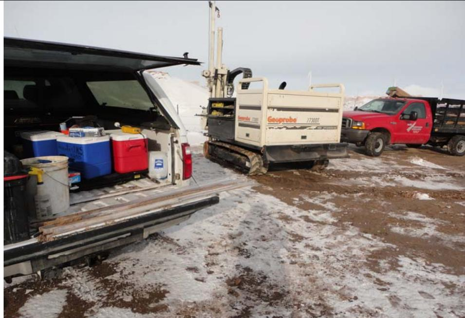
**Subject:** Site Services used a 7730 DT track-mounted Geoprobe® to collect soil samples in Macro-core® barrels containing polyacetate soil sample sleeves.
