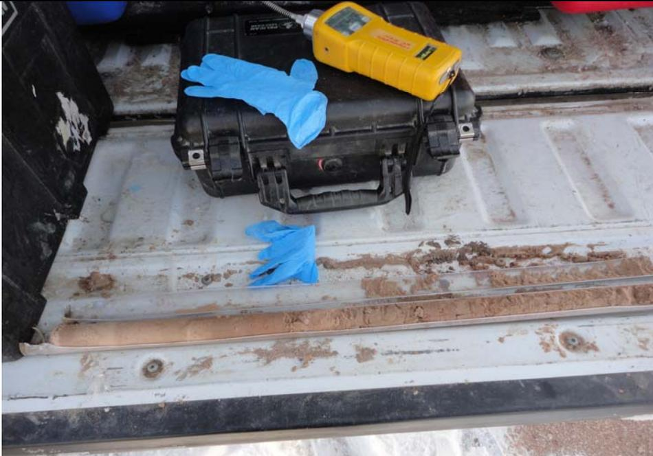
**Subject:** Photograph shows the silty clay lithologies encountered in the test hole that was completed as monitoring well, MW-2. Refusal was encountered at 3 feet bsg, and then again at 12 feet bsg, after augering down using the 3-inch diameter auger. Subcrop consisting of siltstone was observed at the surface.
