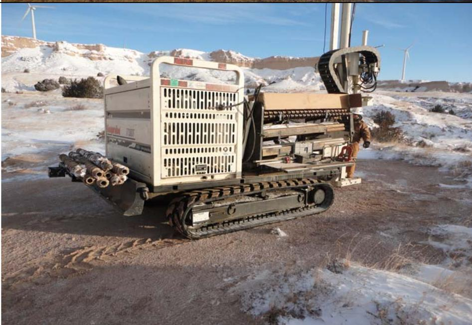
**Subject:** Site Services sets up to probe/drill the test hole for MW-2 using a rubber track mounted 7730 DT Geoprobe® rig.
