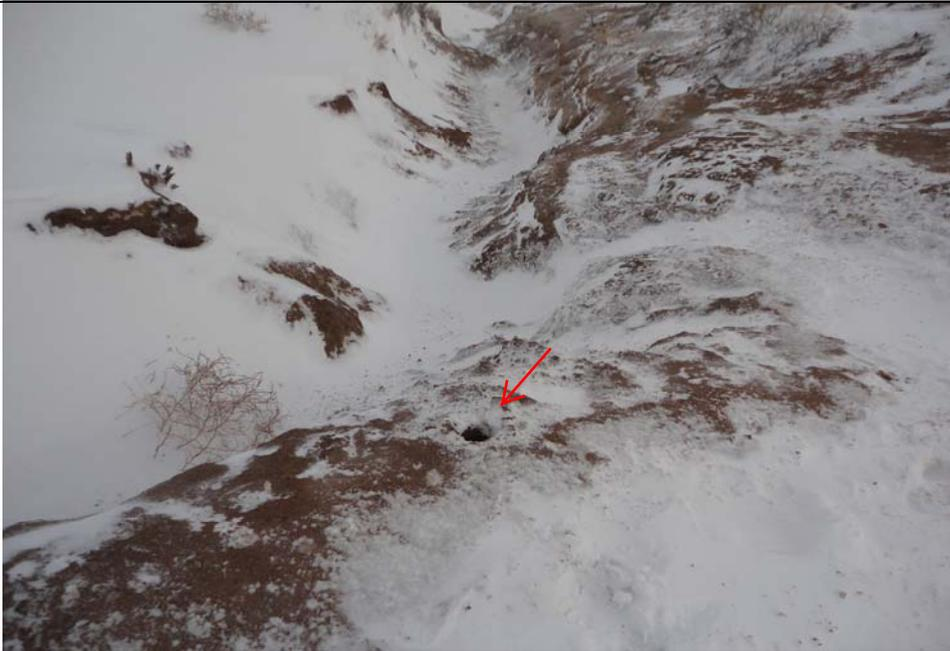
**Subject:** Photograph shows the location of hand auger boring, HA-2, (lower center) at the head of the east-west lateral drainage. Auger refusal was encountered at approximately 4.5 feet. The first hand auger boring, HA-1, was attempted on the lower bench near the center of the photograph, but encountered refusal at approximately 1 foot bsg.
