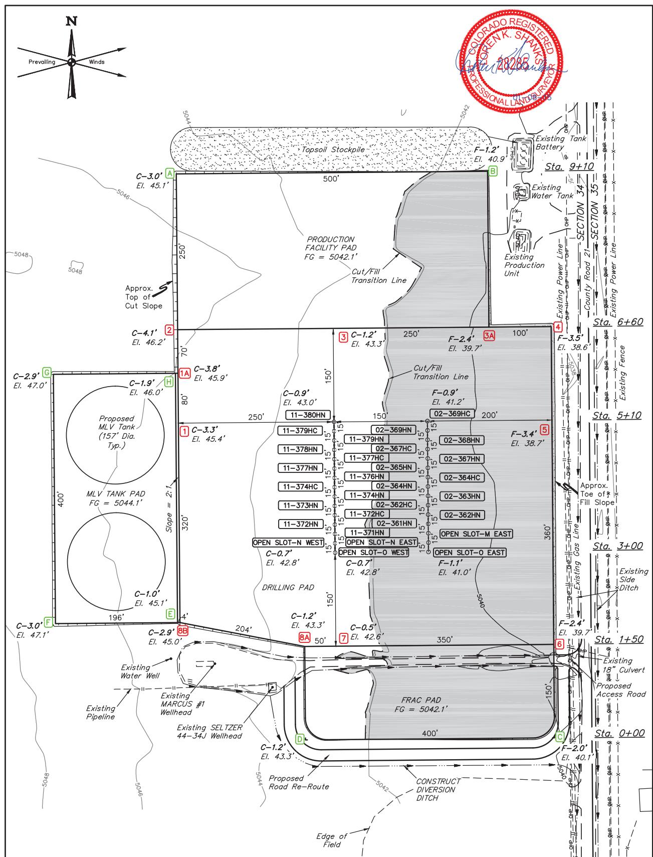
DRILLING PAD FINISHED GRADE ELEVATION = 5042.1'
