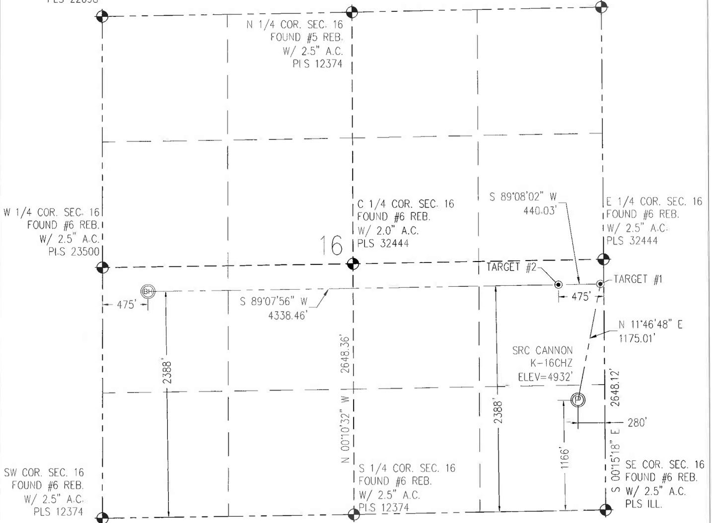
**N** IN ACCORDANCE WITH A REQUEST FROM CRAIG RASMUSON - SYNERGY RESOURCES, BASELINE ENGINEERING CORP. HAS DETERMINED THE LOCATION OF THE SRC CANNON K-16CHZ TO BE 1166' FSL AND 280' FEL, AS MEASURED AT NINETY (90) DEGREES FROM THE SECTION LINE OF SECTION 16, TOWNSHIP 4 NORTH, RANGE 68 WEST AND THE BOTTOM HOLE LOCATION TO BE 2388' FSL AND 475' FWL OF SECTION 16, TOWNSHIP 4 NORTH, RANGE 68 WEST, 6TH PRINCIPAL MERIDIAN, WELD COUNTY, COLORADO.
