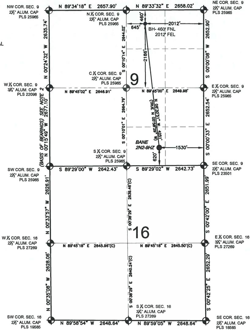
WELL BANE 2N2-9HZ TO BE LOCATED 620' FSL AND 1530' FEL
