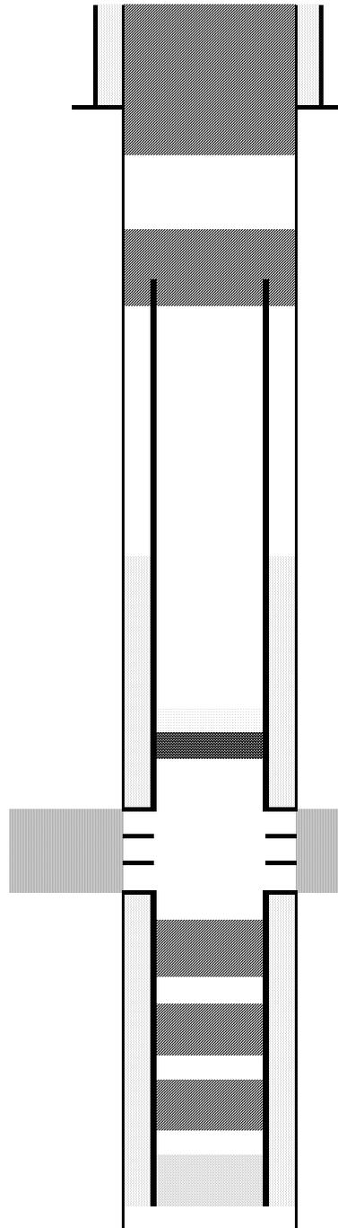
Cut surface casing off 6'-8' below surface.
