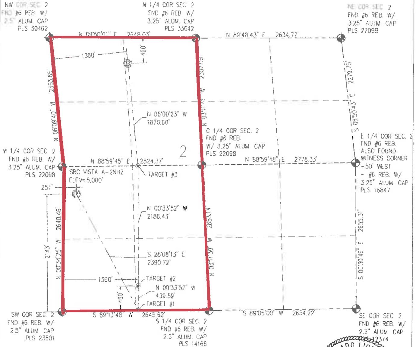
**N** IN ACCORDANCE WITH A REQUEST FROM CRAIG RASMUSON - SYNERGY RESOURCES, BASELINE ENGINEERING CORP. HAS DETERMINED THE LOCATION OF THE SRC VISTA A-2NHZ TO BE 2143' FSL AND 254' FWL, AS MEASURED AT NINETY (90) DEGREES FROM THE SECTION LINE OF SECTION 2, TOWNSHIP 4 NORTH, RANGE 68 WEST AND THE BOTTOM HOLE LOCATION TO BE 460' FNL AND 1360' FWL OF SECTION 2, TOWNSHIP 4 NORTH, RANGE 68 WEST, 6TH PRINCIPAL MERIDIAN, WELD COUNTY, COLORADO
