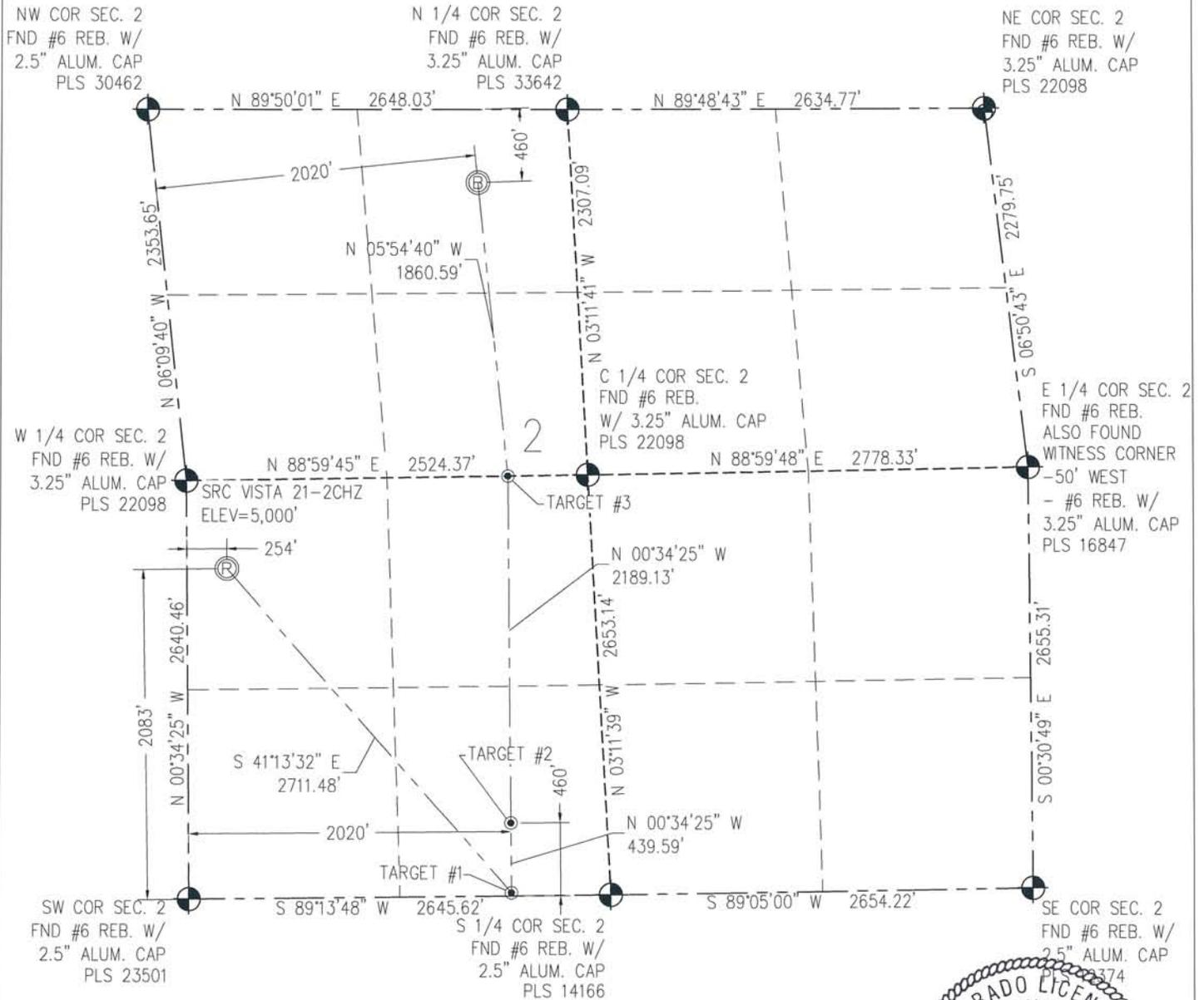
**N** IN ACCORDANCE WITH A REQUEST FROM CRAIG RASMUSON - SYNERGY RESOURCES, BASELINE ENGINEERING CORP. HAS DETERMINED THE LOCATION OF THE SRC VISTA 21-2CHZ TO BE 2083' FSL AND 254' FWL, AS MEASURED AT NINETY (90) DEGREES FROM THE SECTION LINE OF SECTION 2, TOWNSHIP 4 NORTH, RANGE 68 WEST AND THE BOTTOM HOLE LOCATION TO BE 460' FNL AND 2020' FWL OF SECTION 2, TOWNSHIP 4 NORTH, RANGE 68 WEST, 6TH PRINCIPAL MERIDIAN, WELD COUNTY, COLORADO.
