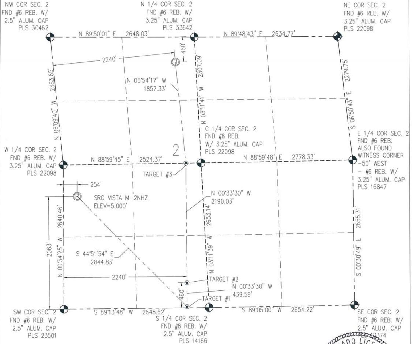
**N** IN ACCORDANCE WITH A REQUEST FROM CRAIG RASMUSON - SYNERGY RESOURCES, BASELINE ENGINEERING CORP. HAS DETERMINED THE LOCATION OF THE SRC VISTA M-2NHZ TO BE 2063' FSL AND 254' FWL, AS MEASURED AT NINETY (90) DEGREES FROM THE SECTION LINE OF SECTION 2, TOWNSHIP 4 NORTH, RANGE 68 WEST AND THE BOTTOM HOLE LOCATION TO BE 460' FNL AND 2240' FWL OF SECTION 2, TOWNSHIP 4 NORTH, RANGE 68 WEST, 6TH PRINCIPAL MERIDIAN, WELD COUNTY, COLORADO.
