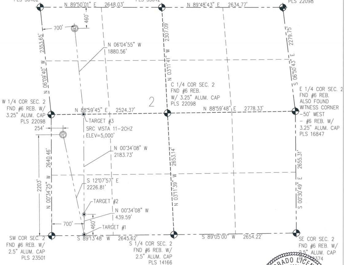
**N** IN ACCORDANCE WITH A REQUEST FROM CRAIG RASMUSON - SYNERGY RESOURCES, BASELINE ENGINEERING CORP. HAS DETERMINED THE LOCATION OF THE SRC VISTA 11-2CHZ TO BE 2203' FSL AND 254' FWL, AS MEASURED AT NINETY (90) DEGREES FROM THE SECTION LINE OF SECTION 2, TOWNSHIP 4 NORTH, RANGE 68 WEST AND THE BOTTOM HOLE LOCATION TO BE 460' FNL AND 700' FWL OF SECTION 2, TOWNSHIP 4 NORTH, RANGE 68 WEST, 6TH PRINCIPAL MERIDIAN, WELD COUNTY, COLORADO.
