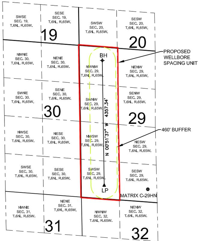
**WELL MATRIX C-29HN TO BE LOCATED 444' FSL AND 2322' FWL, SEC. 29, T6N, R65W**
