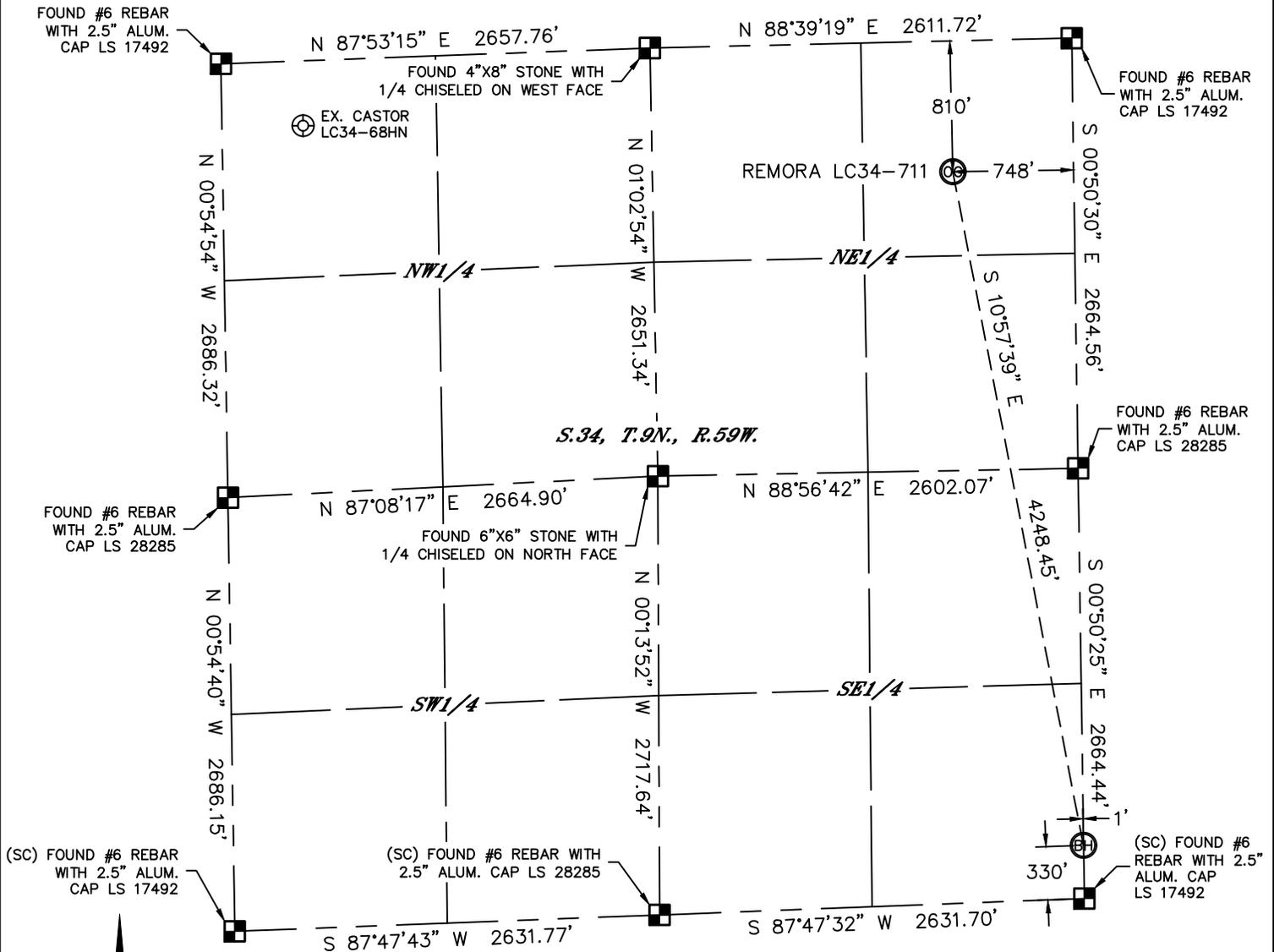
In accordance with a request from Brian James with Noble Energy Inc. Lat40°, Inc. has determined the surface location of the REMORA LC34-711 to be 810' from the NORTH line and 748' from the EAST line and the bottom hole to be 330' from the SOUTH line and 1' from the EAST line as measured at right angles from the section lines of Section 34, Township 9 North, Range 59 West of the Sixth Principal Meridian, County of Weld, State of Colorado.
