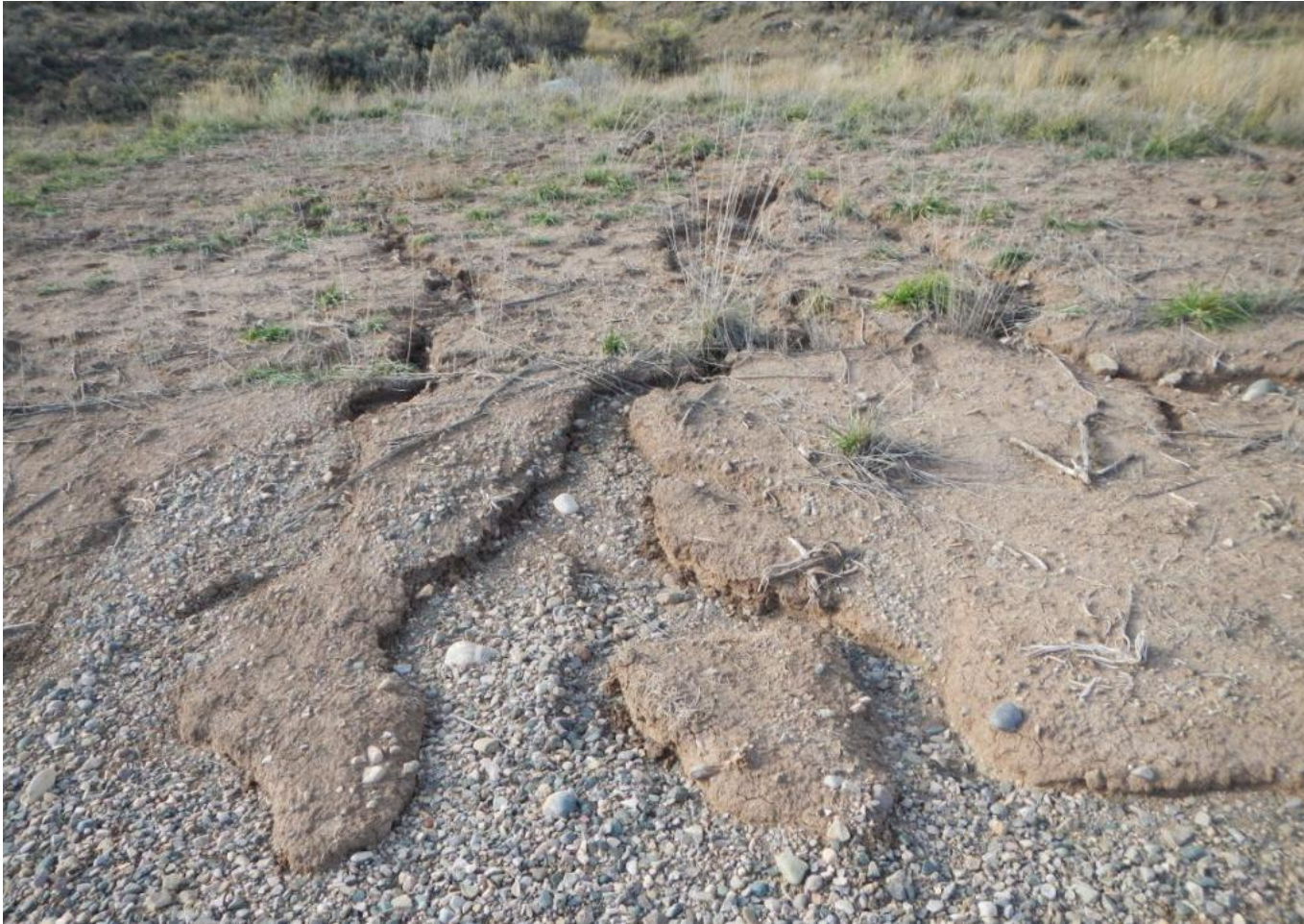
Photo 5. View of rill erosion where there is little revegetation within the interim reclamation area and stormwater exiting the well pad.
