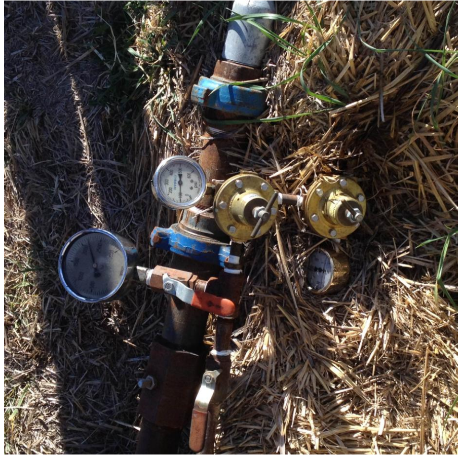
Regulators at time of inspection. 2200 psi on production casing. Two regulators are attached to surface casing. The one to the right read 50 psi.
